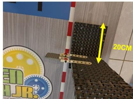
Figure 9.4.1.-5. Top down view of right-hand gantry arm.
