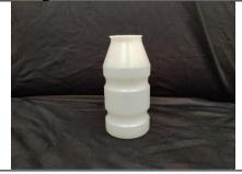
Figure 9.4.2.-4 Image of small bottle, approximately 10.8 cm in height, with a mouth 5.2 cm in diameter, weight 10 grams.
